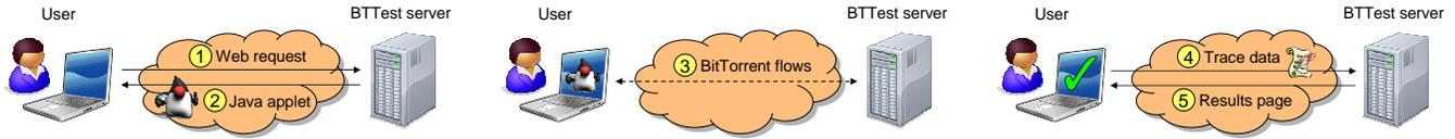
**Figure 1: Overview of the BTTest system:** (1) The user initiates the test. (2) The server sends her a Java applet. (3) The applet connects to the server and emulates a sequence of BitTorrent flows. (4) The applet informs the server whether any flows have been aborted. (5) The server analyzes the information from both endpoints and displays a result page.
